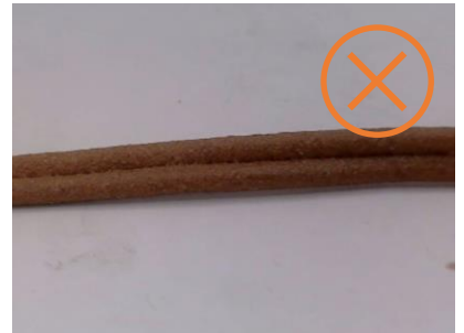
Example 4: „Burnt compound“. This can be caused by too high process temperatures or by a too long residence time in the process.
