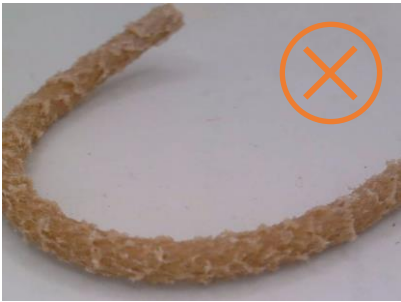
Example 2: Insufficient dispersion of the fibers. This can occur because of a) an inappropriate screw configuration without sufficient mixing zones, b) Insufficient residence time.
