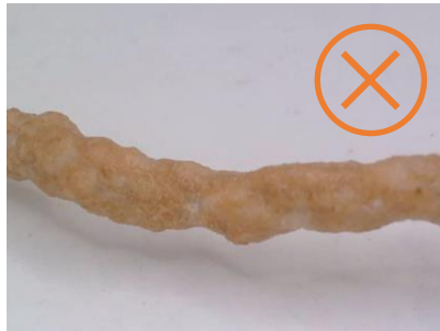
Example 3: Too low process temperatures in the compounder. This results in an inhomogeneous compound with poorly dispersed fibres.
